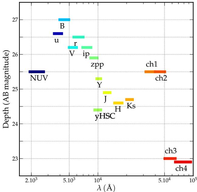
**Figure 3.** Limiting magnitude at  $3\sigma$  in a  $3''$  diameter aperture computed from empty aperture measurements for each band in COSMOS2015, with the exception for NUV filter (value from Zamojski et al. 2007). The length of each segment is the FWHM of the filter curves. For the Y, J, H,  $K_s$  bands; the limiting magnitudes which are specified correspond to  $\mathcal{A}^{\text{UD}}$ .
