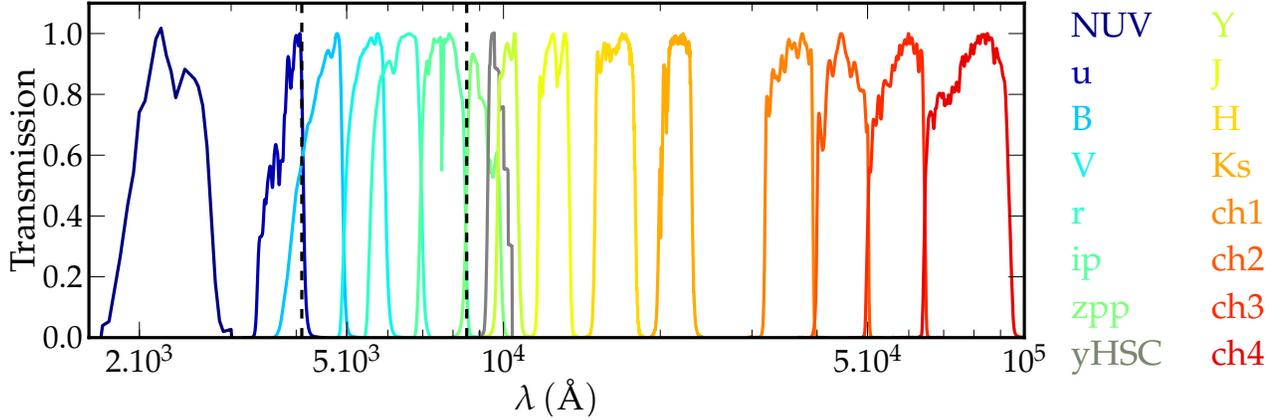
**Figure 2.** Transmission curves for the photometric bands used. The effect of atmosphere, telescope, camera optics, filter, and the detector are included. Note that for clarity the profiles are normalized to a maximum throughput of one: therefore, the relative efficiencies of each telescope and detector system are *not* shown. Intermediate and narrow bands are not represented, but the region of the spectrum covered by these bands is marked by dashed lines.
